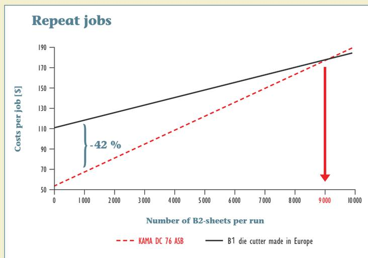
Using of the KAMA DC 76 also makes good sense on repeat jobs. On an order with 2,000 sheets (up to 50,000 cartons depending on size) for example, the cost savings are over 40 %.
